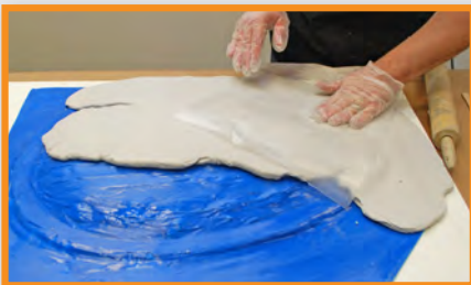
Free Form ® Putty is pressed over a cured Rebound ® 40 rubber mold.
