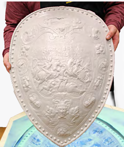
Free Form ® Putty is pressed into a Rebound ® 40 rubber mold of a decorative shield.
