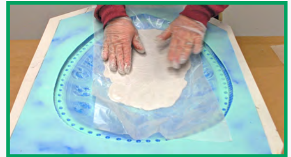
Free Form ® Putty is pressed into a Rebound ® 40 rubber mold of a decorative shield.
