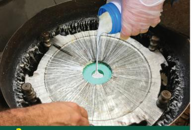
2. Resin is poured into the Smooth-Sil® 960 mold and the mold is spun at a set speed.
