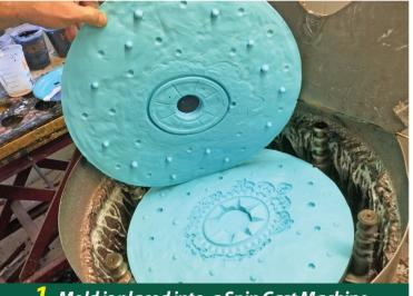
**1.** Mold is placed into a Spin Cast Machine.
