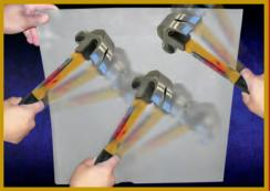
.25 inch panel (.635cm) of Smooth-Cast<sup>®</sup> 45D is semi-rigid, highly impact resistant and easy to bend.
