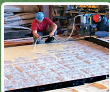
VytaFlex® 60 mold rubber is meter mix dispensed.
