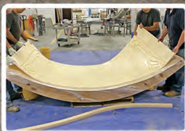
The finished rubber liner is then placed on a concave casting bed.
