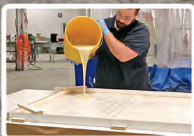
VytaFlex® 60 is properly measured, mixed and poured over the model.
